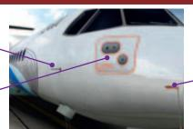
Pitot probe and cover: check, removed
