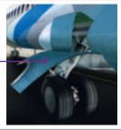
Landing gear structure: check, no crack, no oil
